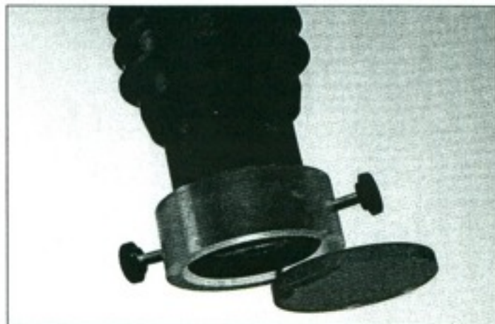
Figure 1: An operator light filter made of orange acrylic filters out light frequencies that would prematurely polymerize light-cured adhesives.
